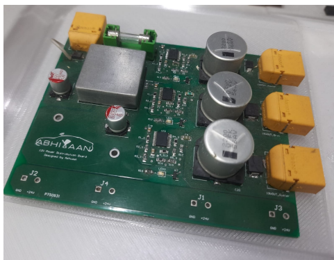
Figure 11: 12 V Power-Protection PCB.
