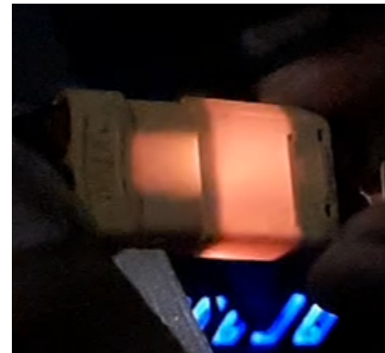
Figure 9: Sparks in XT90 connector without pre-charging.
