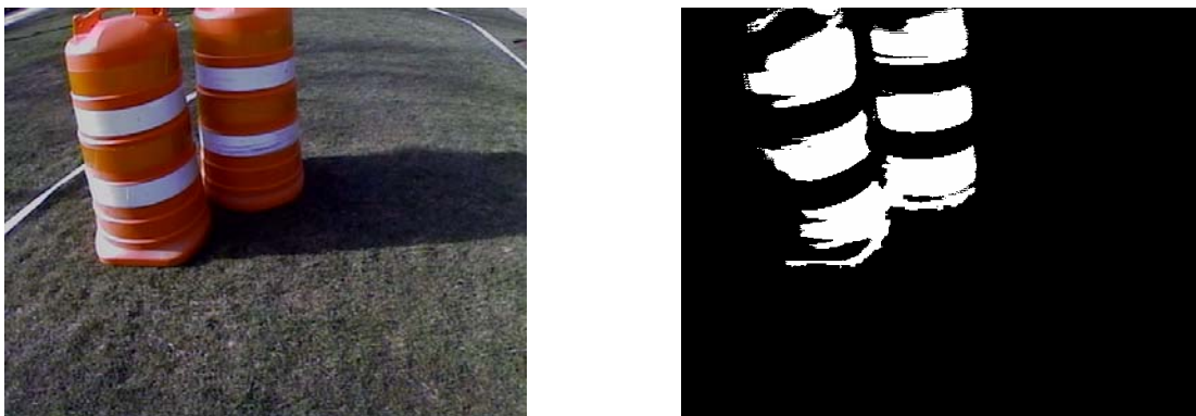
Figure 6: Original and orange barrel segmented image.
