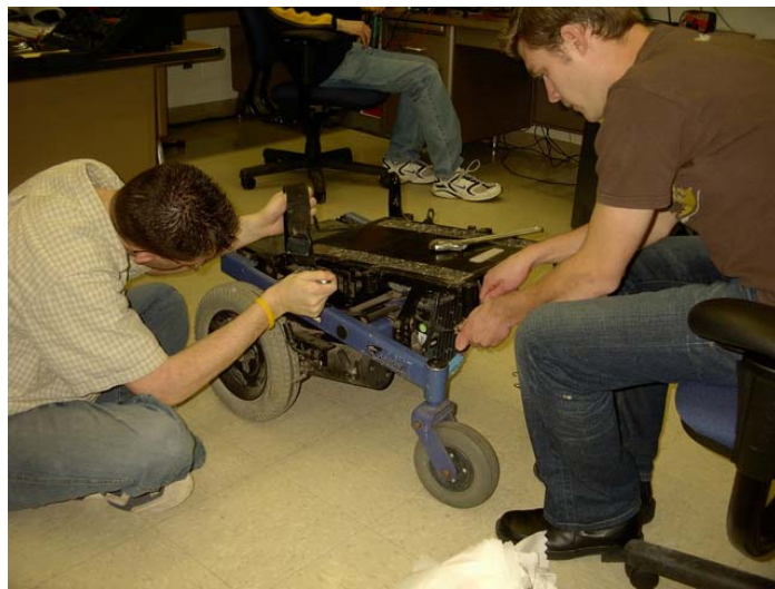
Figure 3: Stripping the chassis of unnecessary parts
