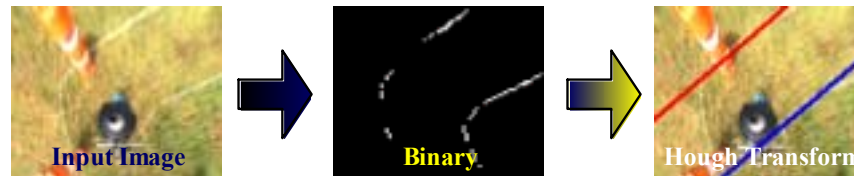
Figure 19: The successful case in which correct lane lines were detected
