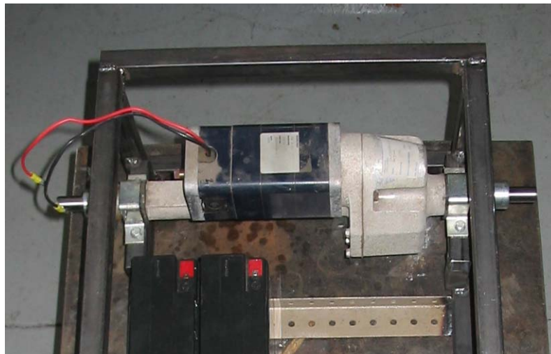
Figure 2: The drive train used in NJAV.
