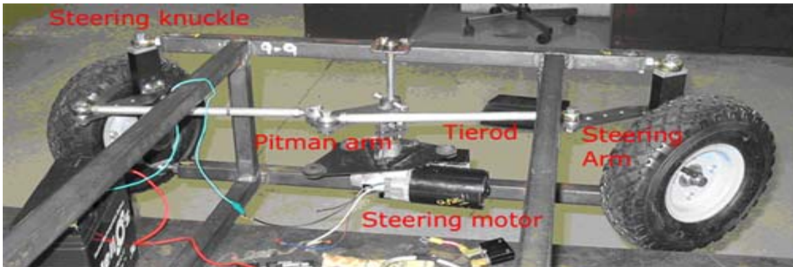
Figure 3: Steering system of NJAV.
