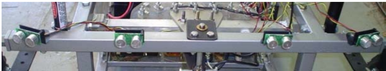
Figure 6: The sensors mounted on the front of the vehicle chassis.
