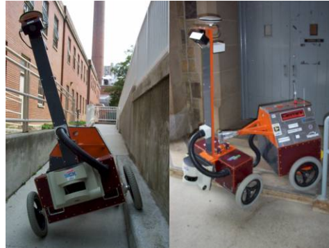
Figure 5: Gemini demonstrating the unique mobility provided by the two degree-of-freedom articulated platform.
