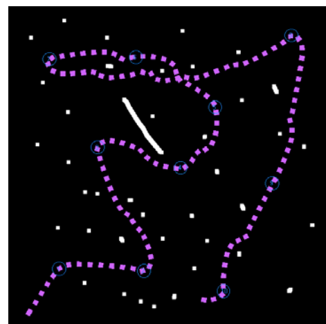
Figure 7.2 Vehicle path (purple), waypoints (blue), obstacles (white) in a simulated IGVC navigation challenge
