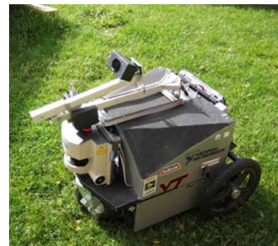
Figure 3.1 Collapsible mast in transport position
