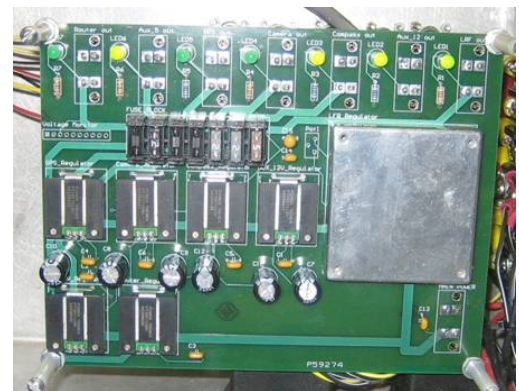
Figure 2: Power distribution board
