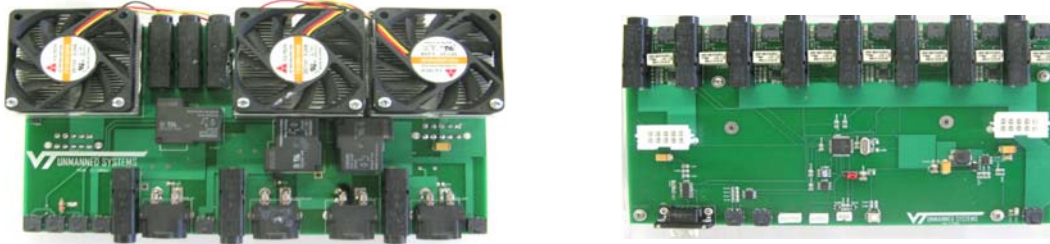
Figure 5.1: Power distribution boards: Input & Regulation (left), Distribution & Monitoring (right)
