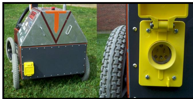
Figure 8: Weatherproof AC power port used for recharging the onboard batteries.
