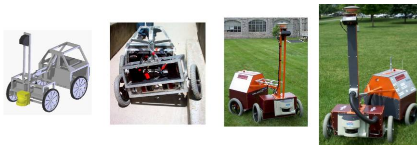
Figure 3: Progression of the design of Gemini from 3-D CAD concept, initial mobility testing, original 2004 IGVC entry, and current configuration for 2006 IGVC entry (left to right).
