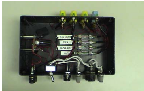
Figure 4.2: The complete Power Supply Module without its cover
