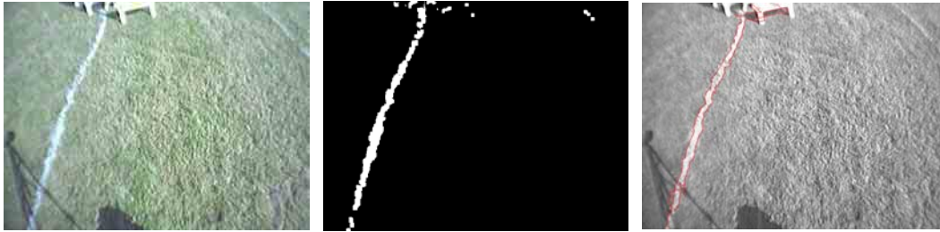
Figure 20 – Image processing steps involved in line detection
