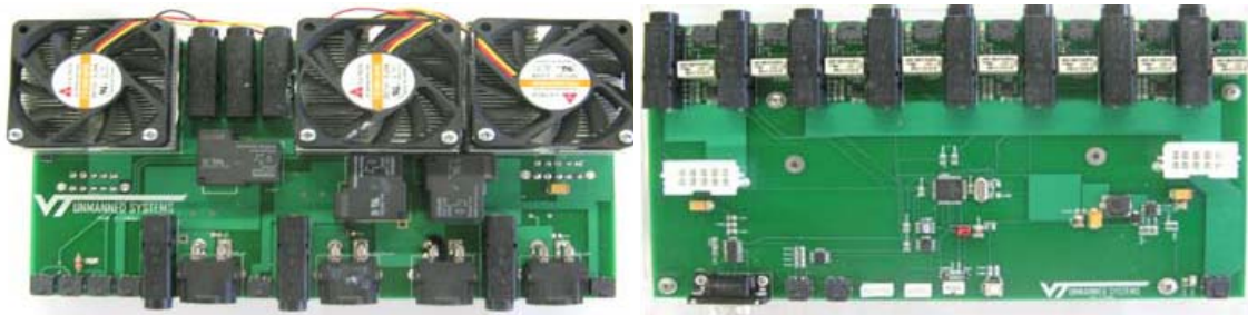
Figure 5.1: Power distribution boards: Input & Regulation (left), Distribution & Monitoring (right)
