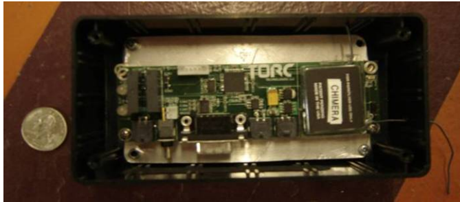
Figure 5.4: RC receiver shown with a quarter for sizing
