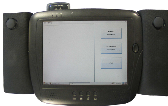
Figure 9-1: Operator Control Unit
