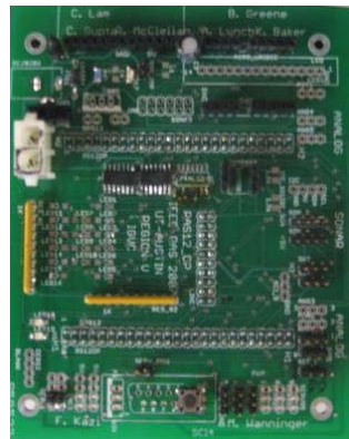
Figure 2: Custom microcontroller PCB for S12
