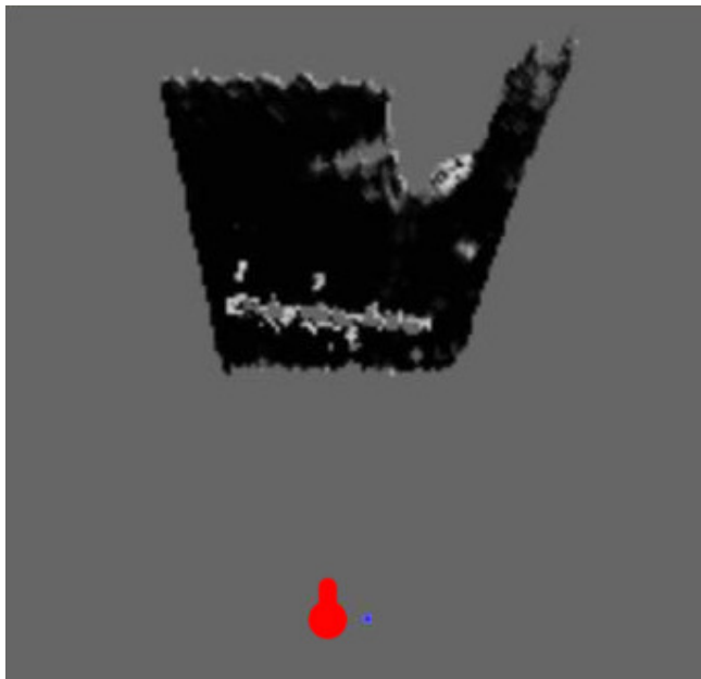
Figure 5: Cost Map resulting from Figure 4. The robot is in red, facing the top of the image. Brighter areas represent higher cost.
