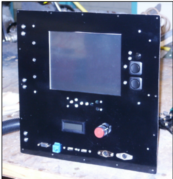
Figure 2 – Revised Control Panel
