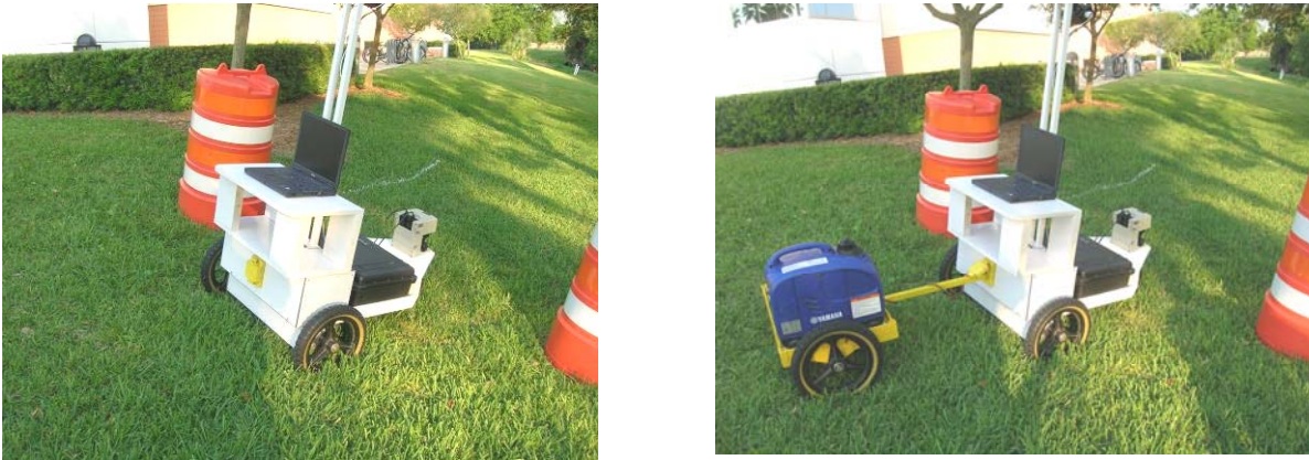
Figure 1.4: Reagle without (left) and with (right) Hybrid-Electric Conversion Trailer
