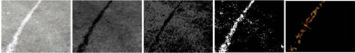
Figure 3. Image Processing Operations for Lane Detection
