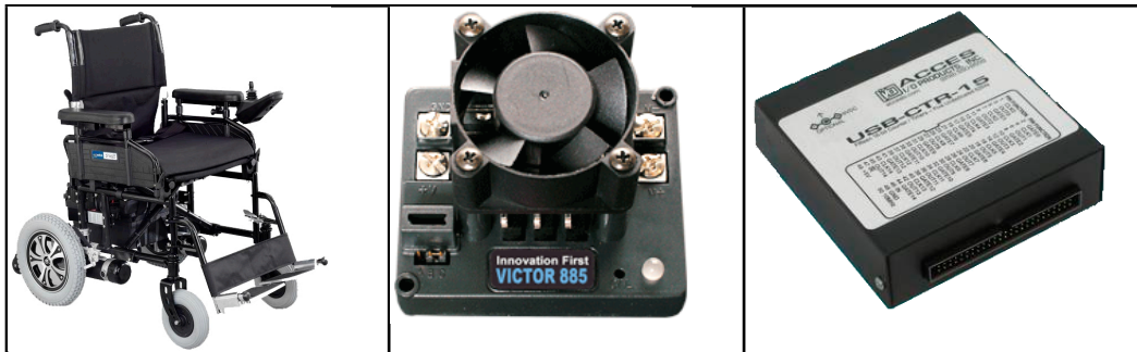
Figure 3. Spirit power wheelchair (left), Victor 885 speed controller (middle) and Acces USB counter-timer module (right)
