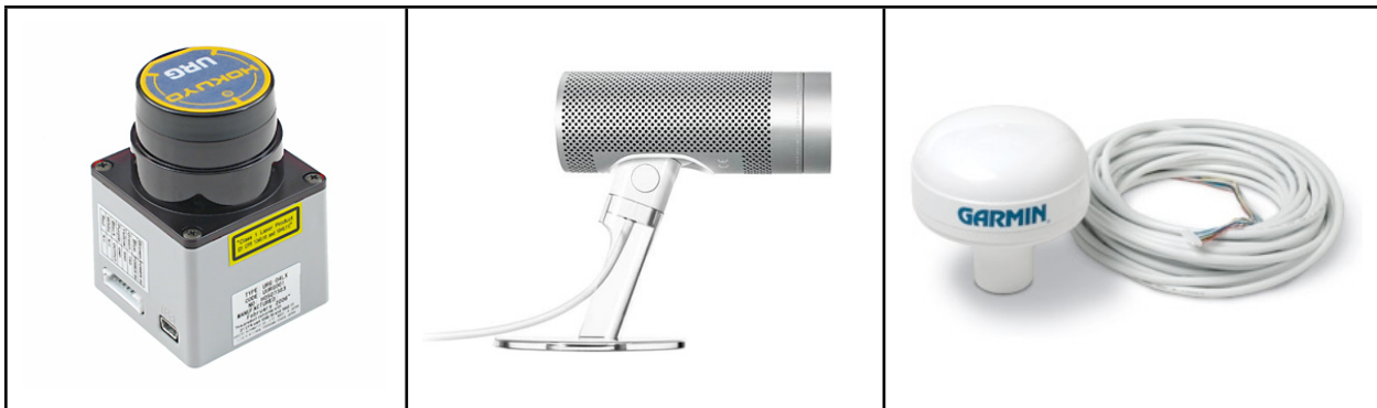
Figure 6. Hokuyo URG-04LX laser scanner (left), Apple iSight digital camera (middle), Garmin GPS 17HVS (right)
