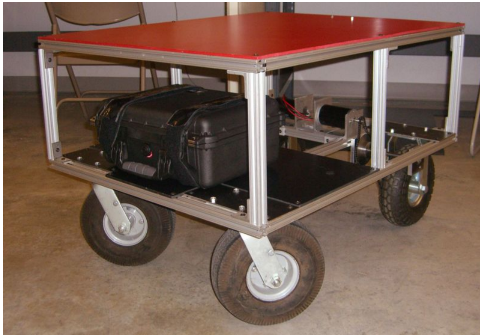
Figure 1: Early chassis, showing the basic structure of the robot
