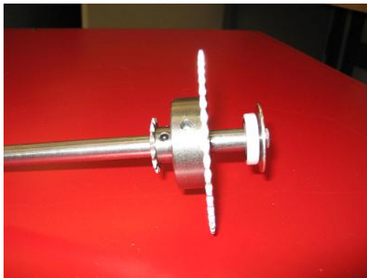
Figure 4: The 72 tooth 5/8" ID sprocket has 4 1/4" holes to mount to the intermediate shaft. The set-up allows for gear balancing to minimize wobble.
