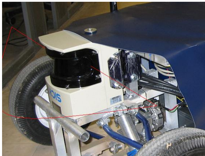
Figure 2-1 - Sick LMS laser range finder showing field of view
