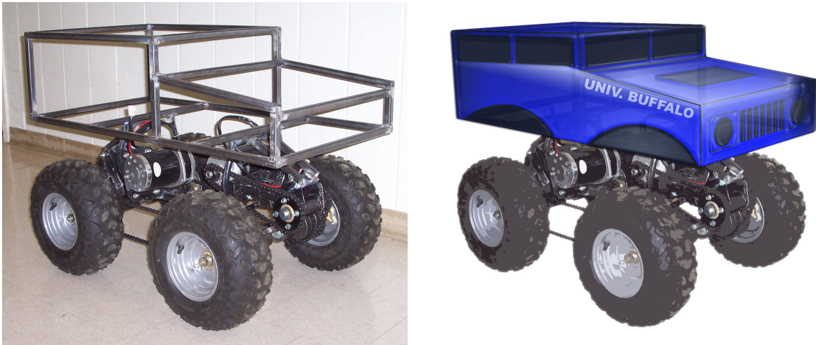
(a) (b) Figure 4.2: Athena's frame and drive train (a) and conceptual body art (b)
