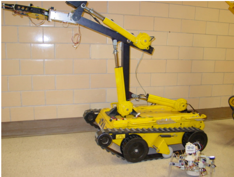
Figure 1 Original Israel Military Industries MK-5 Hornet bomb disposal robot
