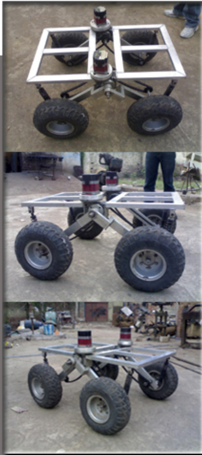
Original Chassis using Aluminum 6063.
