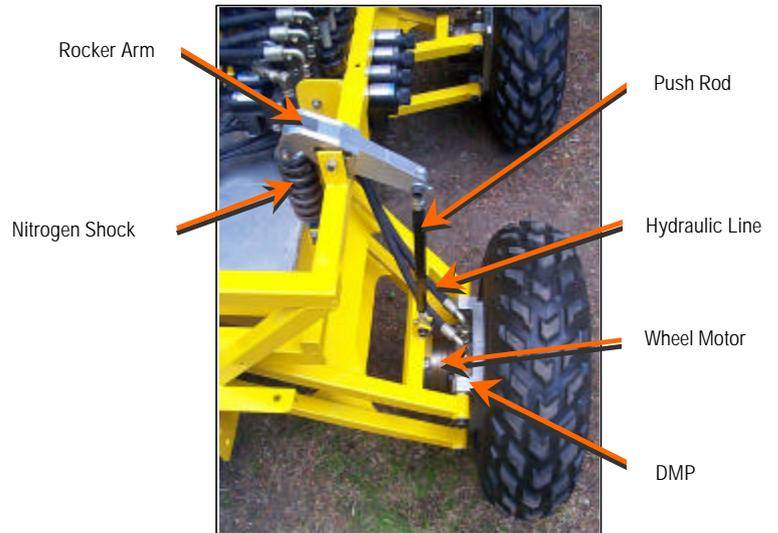
Figure 1 – Mechanical detail.
