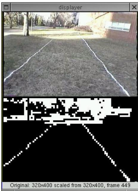
Figure 5a – Original captured image (top) and processed image with reduced resolution (bottom).
