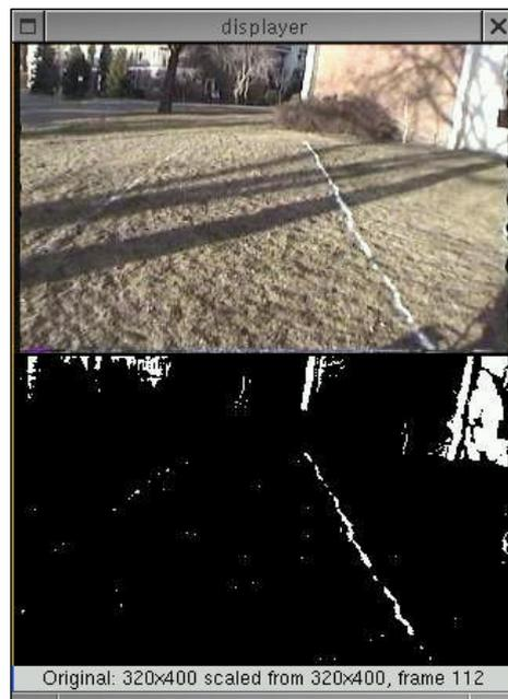
Figure 5b – Original captured image with shadows (top) and processed image (bottom).
