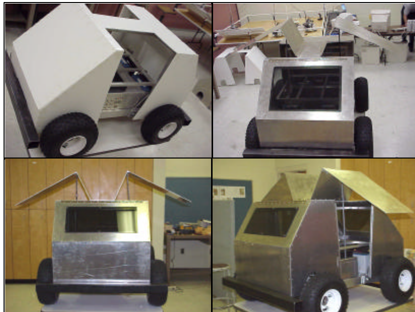
Figure 2. TIGER Body Prototype and Its Final Delorean Style Physical Body.
