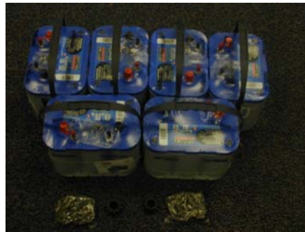
Figure5B: 12V Marine Deep Cycle Batteries
