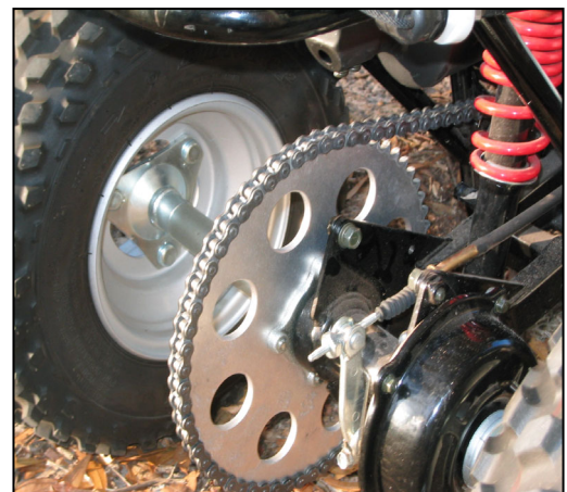
Figure 15 - New Rear Sprocket
