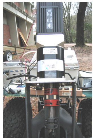
Figure 5 - Steering actuation with slip coupling
