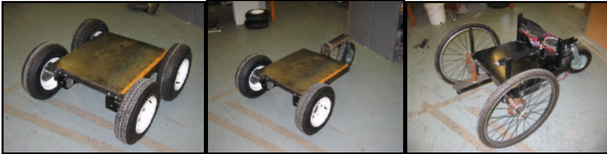
Figure 3.1 – The vehicle base of Optimus in 4-wheel and both 3-wheel configurations
