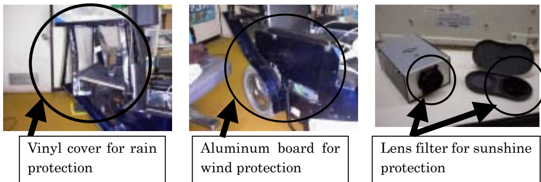
Fig. 5: Proposed protection for the AMIGO 2002
