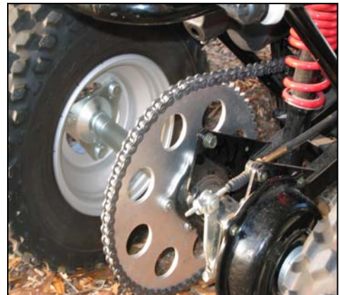
Figure 6 - New Rear Sprocket
