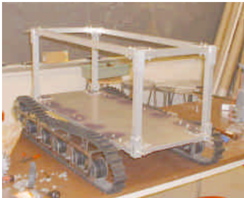
Figure 4: Corner View of Frame and Track
